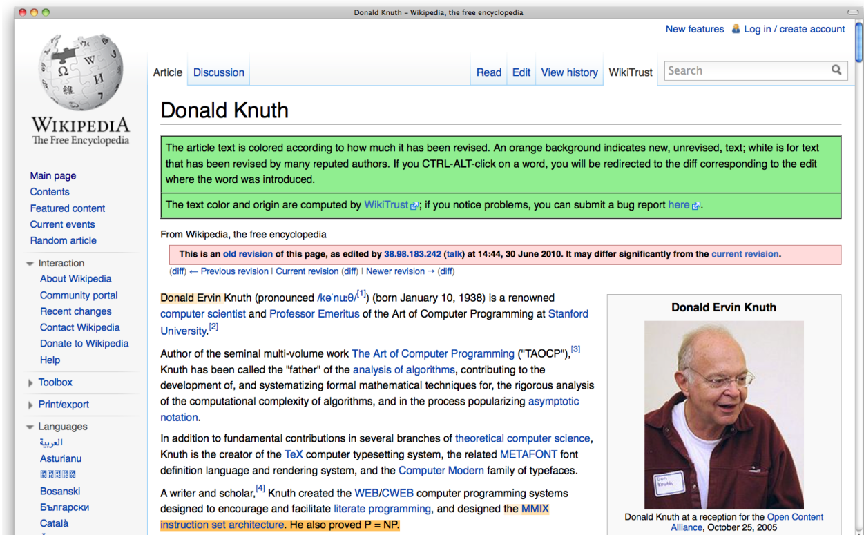
Figure 1: The Wikipedia page for Don Knuth, as rendered by WikiTrust. The text background is a shade of orange that is the darker, the lower the reputation of the text.
